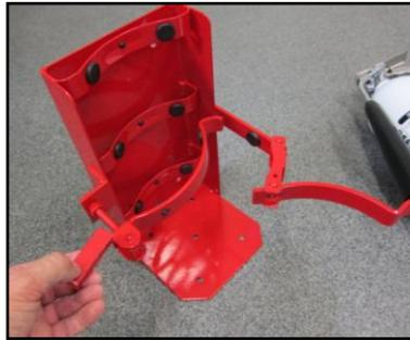
Figure 7. Testing bracket with hand-held magnet
