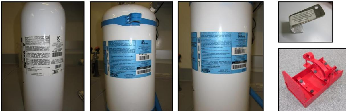
Figures 1-5. Photos of Amerex fire extinguishers and brackets that were examined in MRI fringe magnetic field.
